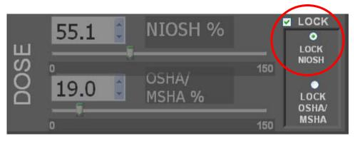
Note that if a <u>SOUND LEVEL THRESHOLD</u> (80 dBA or 90 dBA) has been selected in the <u>USER PREFERENCES</u> menu, the LOCK checkboxes are disabled, preventing back-calculating (since setting a SOUND LEVEL THRESHOLD creates a discontinuity in the equation used to calculate the DOSE, making back calculation impossible in
