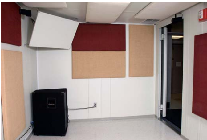
Fig. 4 - Test chamber interior. a) A hard-walled test chamber with diffuser panels (shown in “auditory demonstrations mode” with removable absorptive wall panels) provides a low-noise reverberant environment for hearing protector evaluation. b) Hearing protector evaluations on human subjects seated in the test chamber are conducted from the control console by means of a visualization window and two-way communication system.
