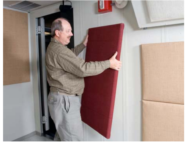
Fig. 3 - Hearing protector evaluation. a) Control console includes equipment racks for hearing protector testing (left) and auditory demonstrations (right). b) Removable absorptive wall panels allow the chamber to be reconfigured as a free-field room for developing and presenting auditory demonstrations.
