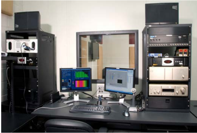
Fig. 3 - Hearing protector evaluation. a) Control console includes equipment racks for hearing protector testing (left) and auditory demonstrations (right). b) Removable absorptive wall panels allow the chamber to be reconfigured as a free-field room for developing and presenting auditory demonstrations.
