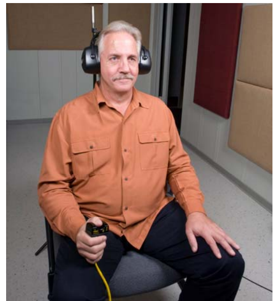
Fig. 4 - Test chamber interior. a) A hard-walled test chamber with diffuser panels (shown in “auditory demonstrations mode” with removable absorptive wall panels) provides a low-noise reverberant environment for hearing protector evaluation. b) Hearing protector evaluations on human subjects seated in the test chamber are conducted from the control console by means of a visualization window and two-way communication system.
