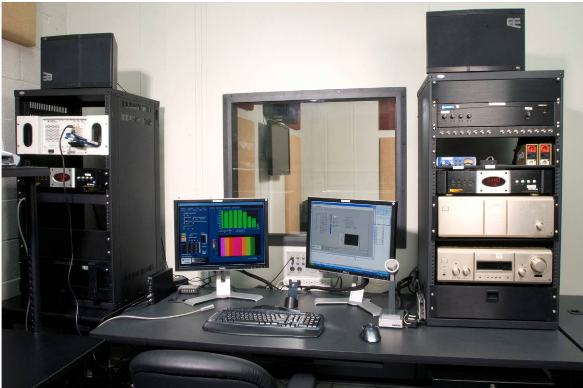
Figure 2 – NASA GRC Auditory Demonstration Laboratory control room with NASA REATMaster and Stimulus Presentation Sound System Rack (left) and Auditory Demonstrations Rack (right)
