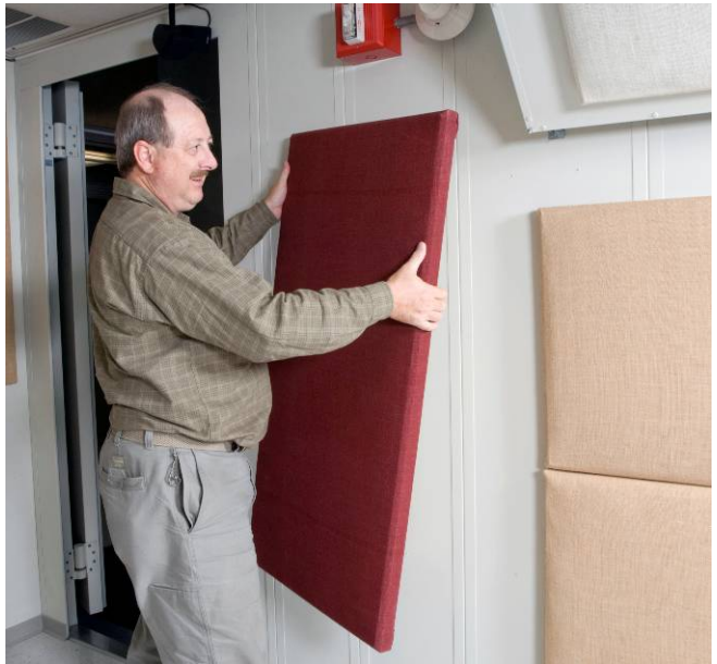
Figure 5 – The fabric panels in the ADL test chamber are removed from the test chamber when it is used for REAT testing. The fabric panels add the absorption needed to make the chamber convertible for use in presenting auditory demonstrations using the secondary audio sound system.
