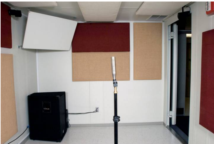
Figure 4 – Interior view of NASA GRC Auditory Demonstrations Laboratory REAT test chamber, showing ElectroVoice speakers, diffusing panels and GRAS low noise microphone system used for background noise measurement.
