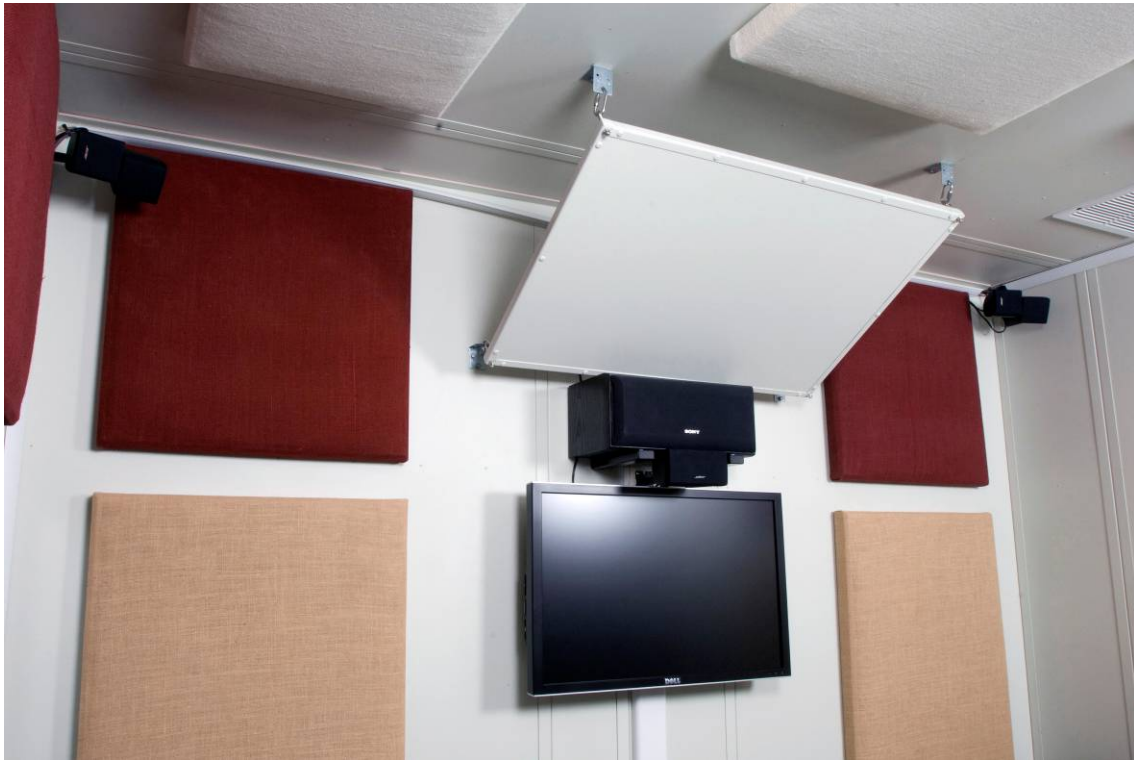
Figure 3 – Interior View of NASA GRC Auditory Demonstrations Laboratory REAT Test chamber, showing diffusing panel, intercom speaker system and subject instruction video display
