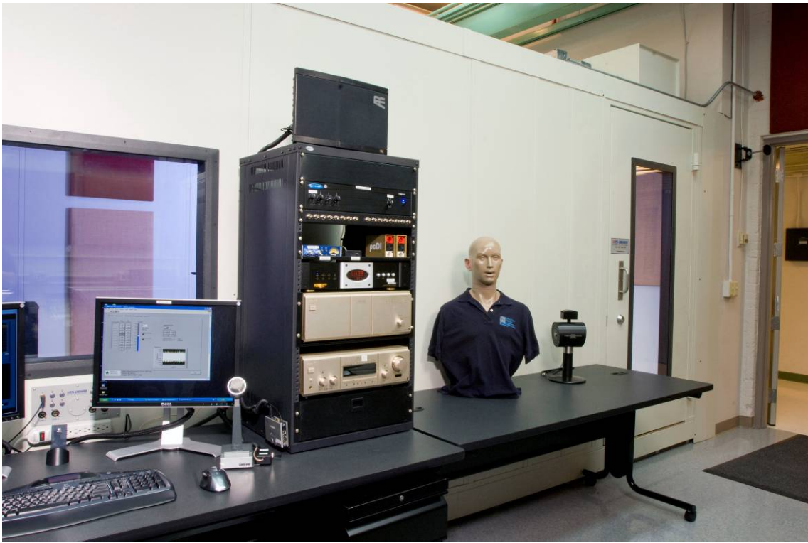
Figure 1 – Exterior View of the NASA GRC Auditory Demonstrations Laboratory Real Ear Attenuation test chamber, control space and test fixtures.
